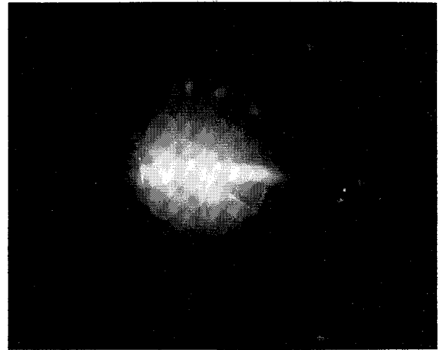
Fig 5 Photograph of plasmajet at higher flow rate (argon gas at 1 atm) Flow rate, 30 g/min; voltage, 32 v; current, 105 amps
